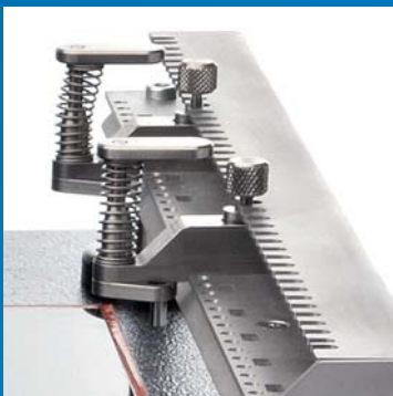
Practical clips for especially large printed circuit boards
