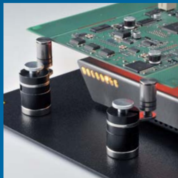
Height adjustable clamps Handy Fix 06 with 4 magnetic holders
